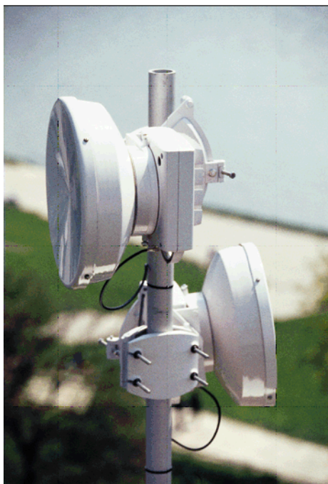
Figure 1. Nokia FlexiHopper outdoor unit
